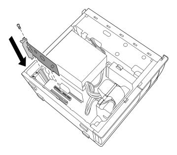
5 Replace the screw that secures the card.
